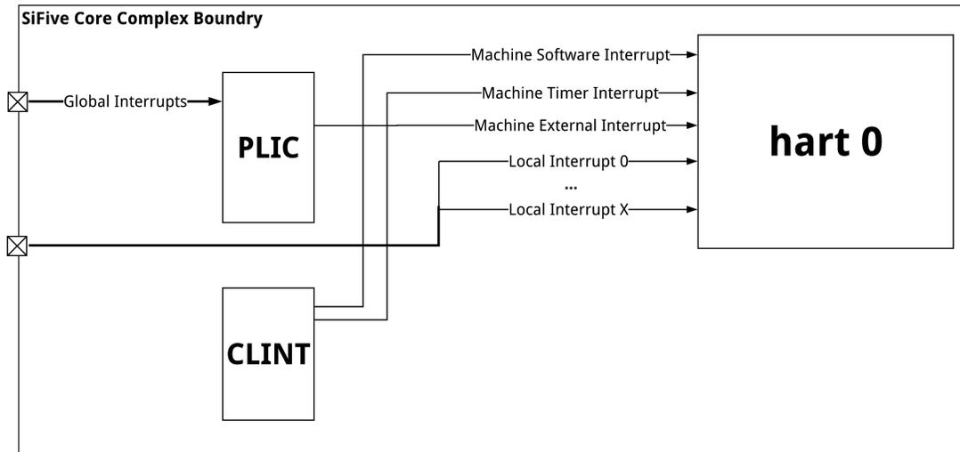
**Figure 2:** E34 Core Complex Interrupt Architecture Block Diagram.
